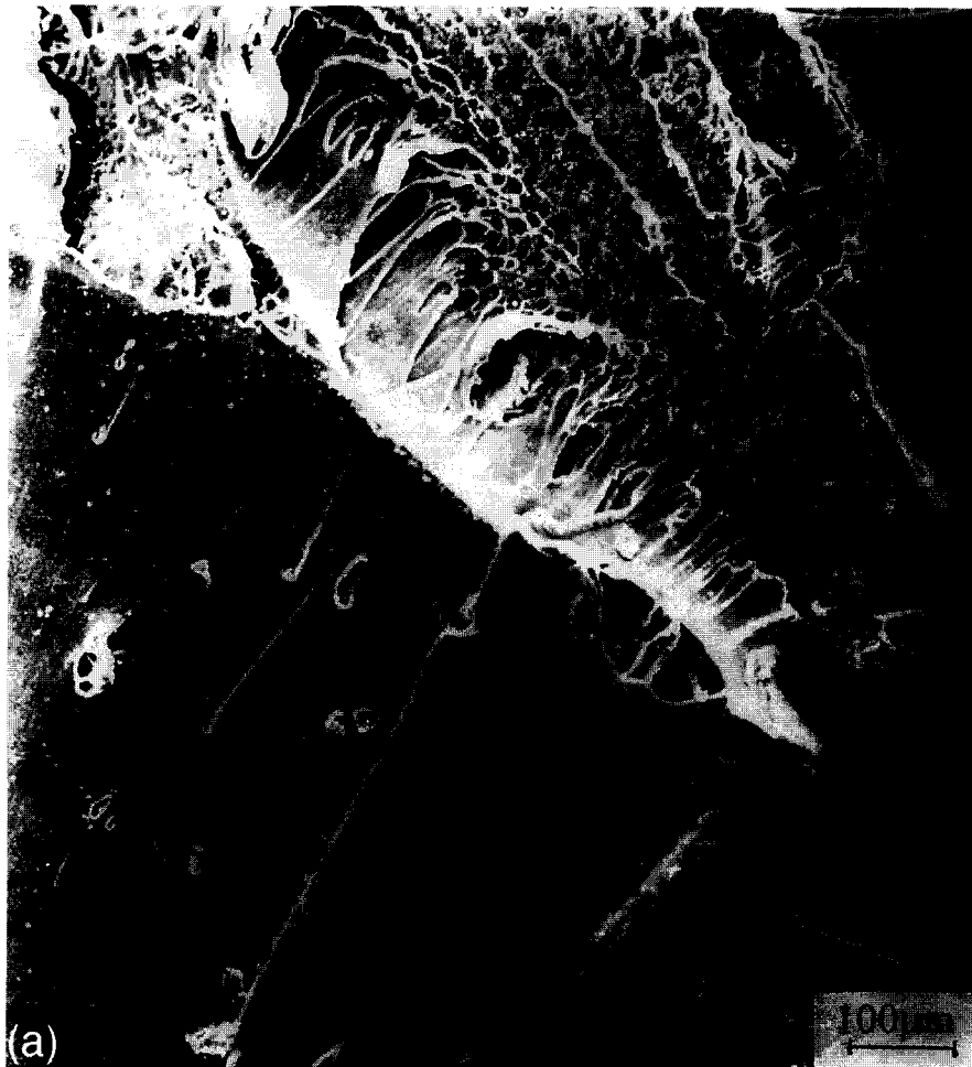
Figure 6 Higher magnification view of the stable-unstable transition on the fatigue fracture surface. (a) S_{\max} = 0.9 UTS, R = 0.1 ; (b) S_{\max} = 0.4 UTS, R = 0.1 ; (c) S_{\max} = 0.5 UTS, R = 0.3
