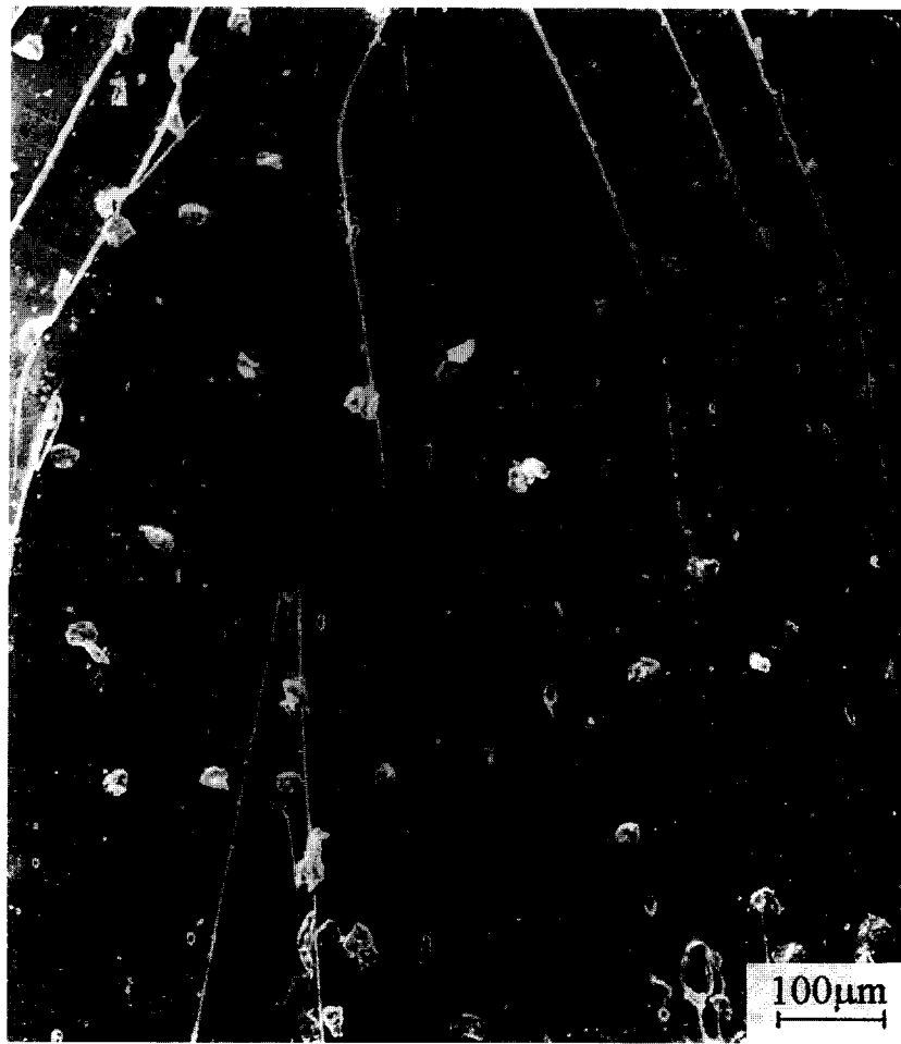
Figure 3 Higher magnification view of crack slow-growth region at point A of Figure 2
